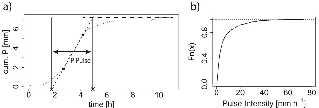
**Figure 2.** (a) Example of cumulative rainfall (cum. P) with time used for the transformation of a rainfall event to a rain pulse and (b) the resulting empirical cumulative density function of intensities for every infiltration event with rainfall duration  $\leq 3$  h.
