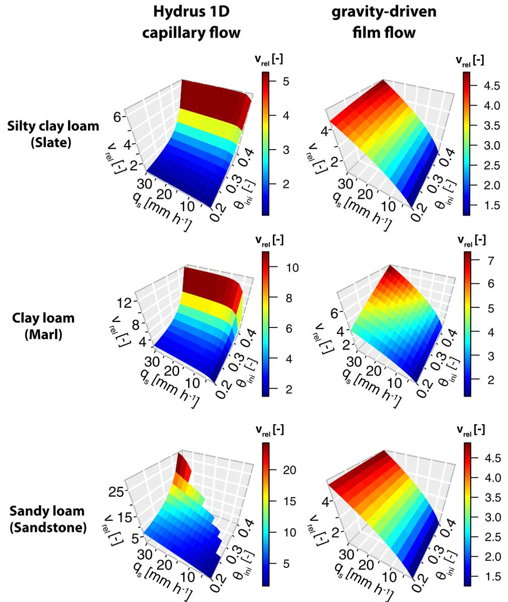
**Figure 7.** Comparison of relative increase in modeled wetting front velocities ( $v_{rel}$ ) with rainfall pulse intensity ( $q_s$ ) and initial water content ( $\theta_{ini}$ ) for the film flow and capillary flow (HYDRUS 1D) approach. Comparison was done for the three geologies of the grassland sites at 30 cm depth.
