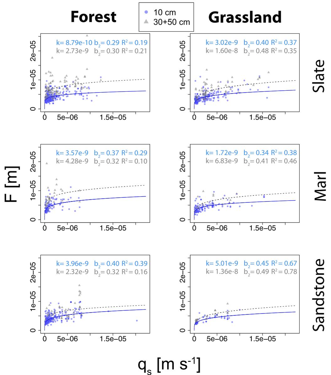
**Figure A2.** Relationships of the rainfall intensity ( $q_s$ ) and the film thickness ( $F$ ) as presented in Equation A3.
