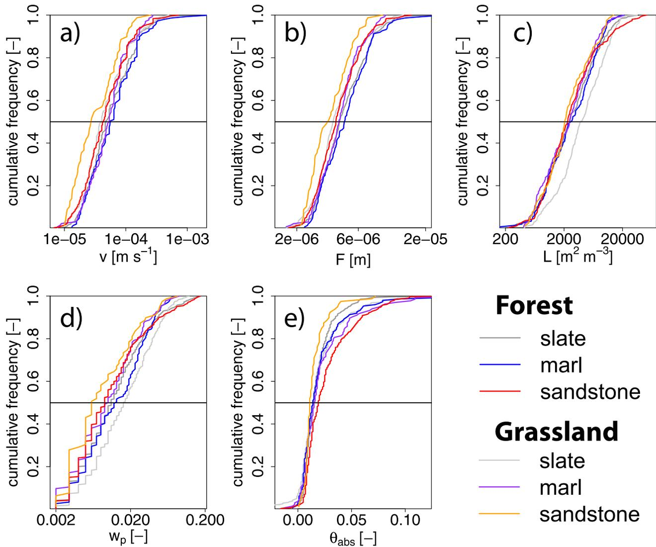
**Figure 4.** Empirical cumulative distribution of the parameters extracted from the WCWs (optimization) showing (a) the wetting front velocity  $v$ , (b) film thickness  $F$ , (c) specific contact area  $L$ , (d) peak mobile water content  $w_p$  and (e) water abstraction by the soil matrix  $\theta_{abs}$ . WCW, water content wave.
