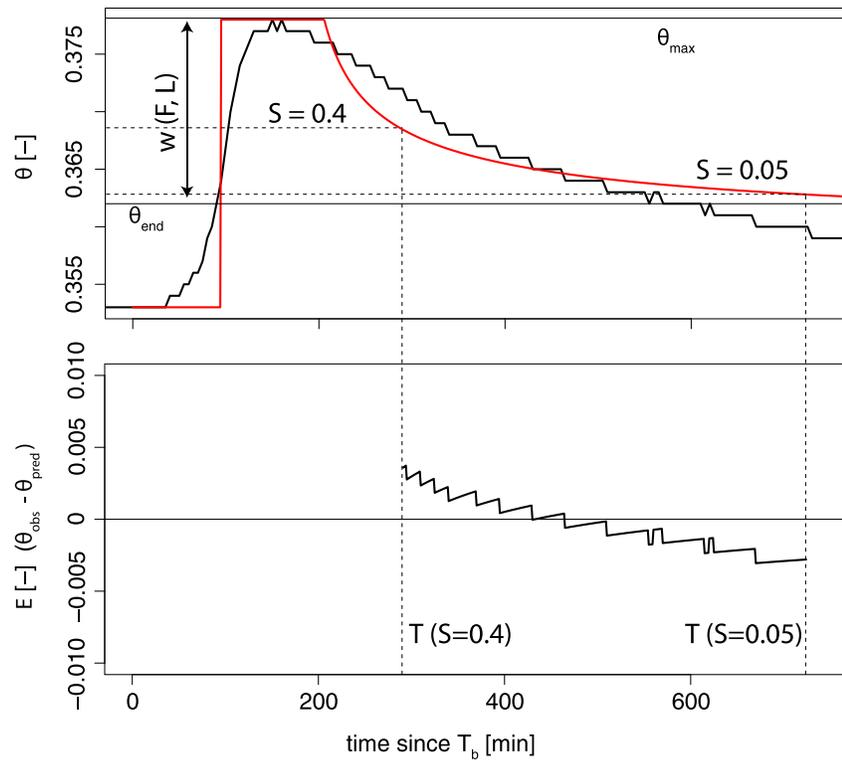
**Figure 3.** Schematic diagram showing the definition of the termination criterion based on the parameter  $S$  (upper plot) and the resulting error in soil water content (lower plot) representative for one WCW. In the upper plot the black line illustrates the observed data ( $\theta_{\text{obs}}$ ) whereas the red line shows the optimized WCV ( $\theta_{\text{pred}}$ ). WCW, water content wave.
