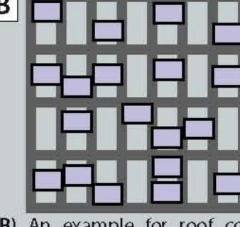
B) An example for roof coverage of 45 %. The roofing elements are moved randomly every month according to needed coverage.
