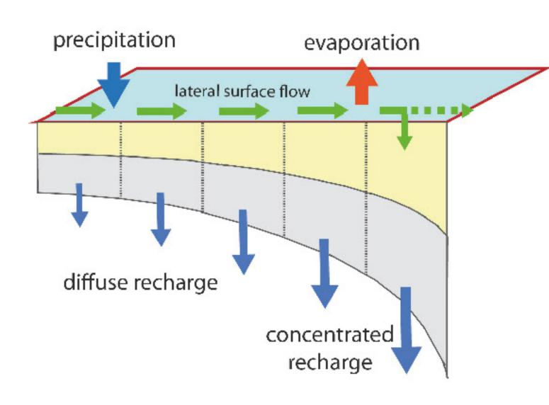
We simulate groundwater recharge with a semi-distributed model that considers the spatial heterogeneity of the karst system by distribution functions.
