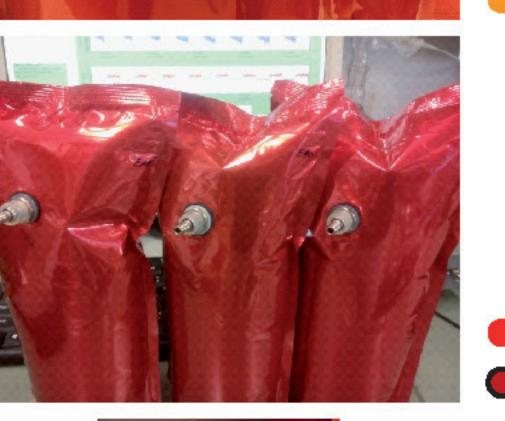
3-layer metalized ziploc bags. Commercially available gasvalves applied for filling and sampling via tubing.
