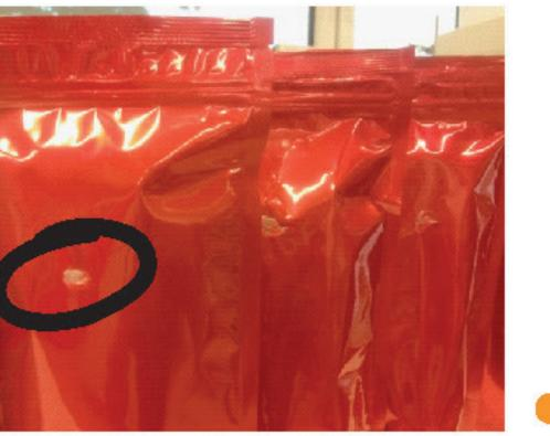
3-layer metalized ziploc bags. Silicone blot serves as septum Filling and sampling through septum via needle and 1/8" tubing.
