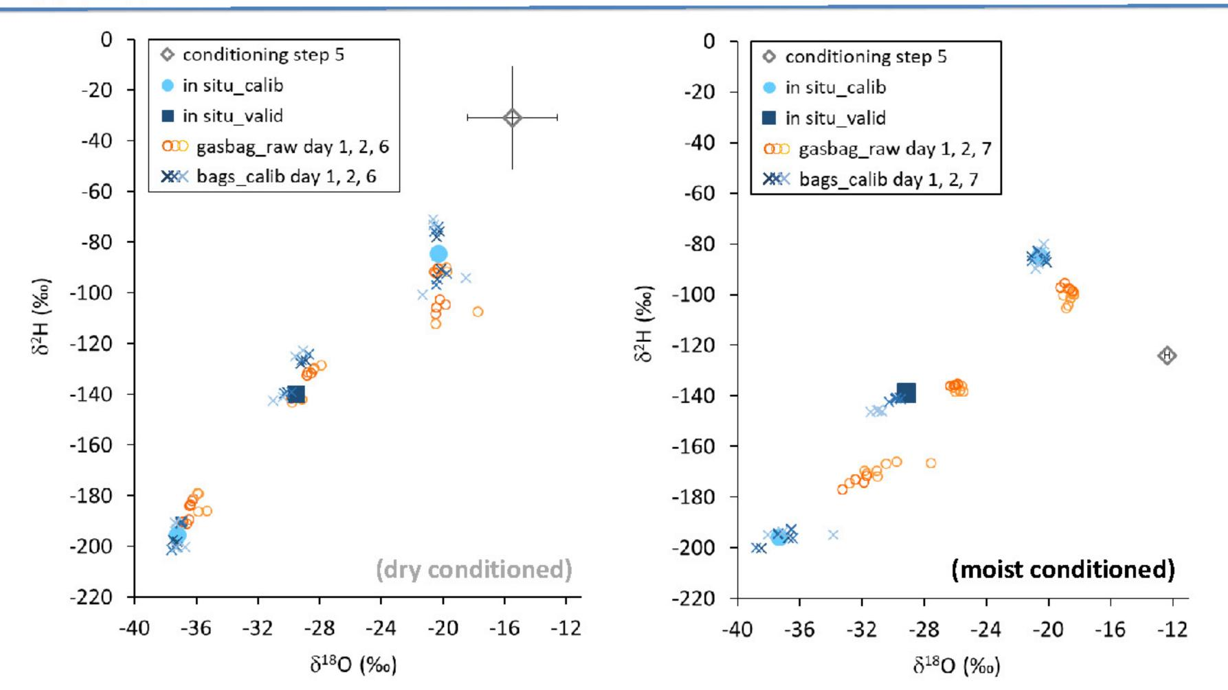
Repeated bag measurements (1, 2, 7 days) from sampling of three different isotopic reservoirs. Sampling bags were conditioned with dry (left) and moist (right) atmosphere. *In situ* measurements (filled symbols) were more reliably calculated from moist than from dry conditioned bag measurements (crosses). Pre-sampling measurements are shown as gray open diamonds. Note that their error bars (black) are smaller than the symbol, in the case of moist conditioning.
