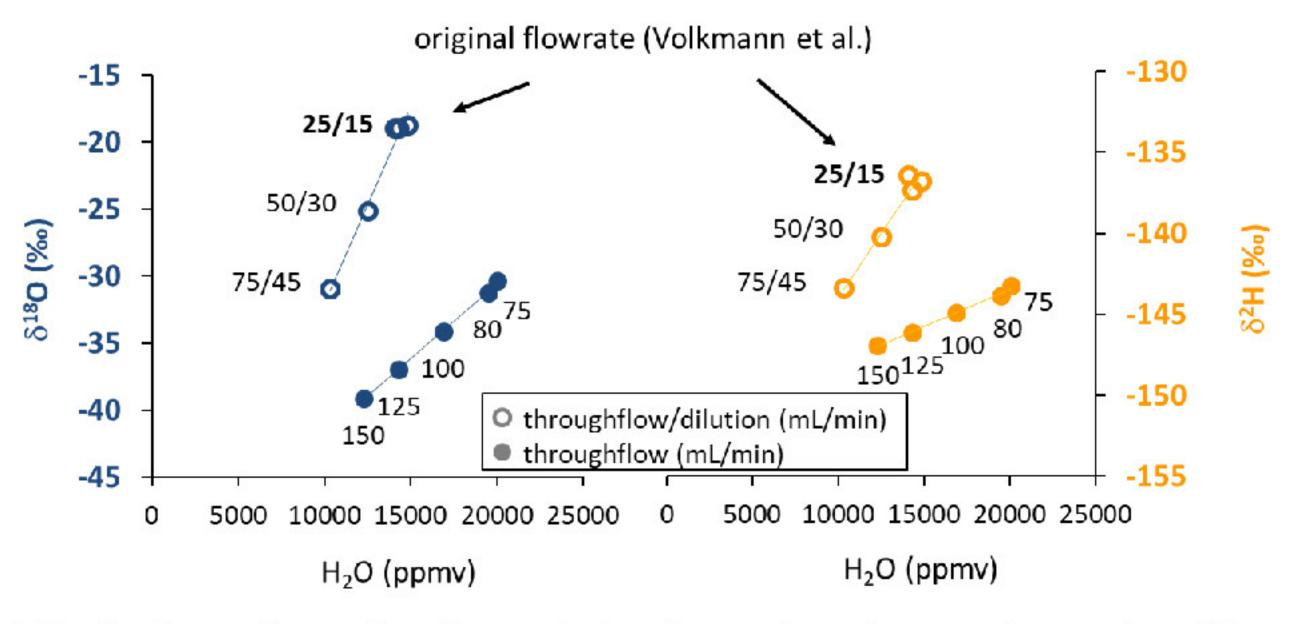
Effect of gas flowrates through in situ probes (increased, to reduce filling time of bags): Decrease of water vapor content and depletion in isotopes (left:  $\delta^{18}$ O, right:  $\delta^{2}$ H) is obtained by increasing gas flowrates with (open symbols) and without (closed symbols) dilution, due to incomplete equilibrium. Numbers refer to the respective gas flowrates applied: throughflow/dilution or throughflow-only.
