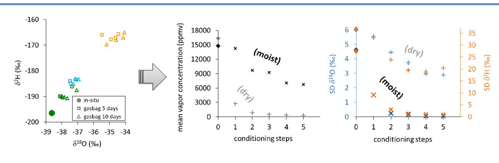
(left) Vapor content and standard deviations (SD) of vapor isotopes (right) from a batch of bags, stepwise conditioned with synthetic air (light plus symbols) and moist air (dark symbols). Diamond symbols on vertical axes represent respective mean values of pre-conditioning measurements
