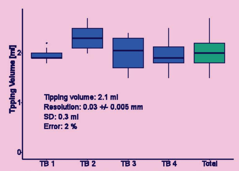
The accuracy test of the TB shows small differences among the different TBs due to unevenness caused by the 3D printer. Compared to other TBs installed in rain gauges the accuracy is comparable and acceptable.
