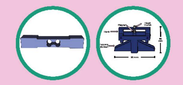
The load cells (LC) have a resolution of 6 g. After calibration, they show good accuracy.
